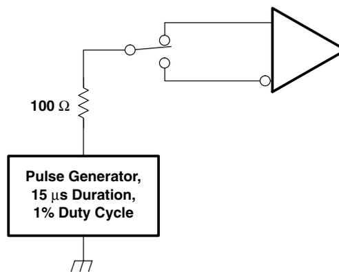
Figure 7. Overvoltage Protection
